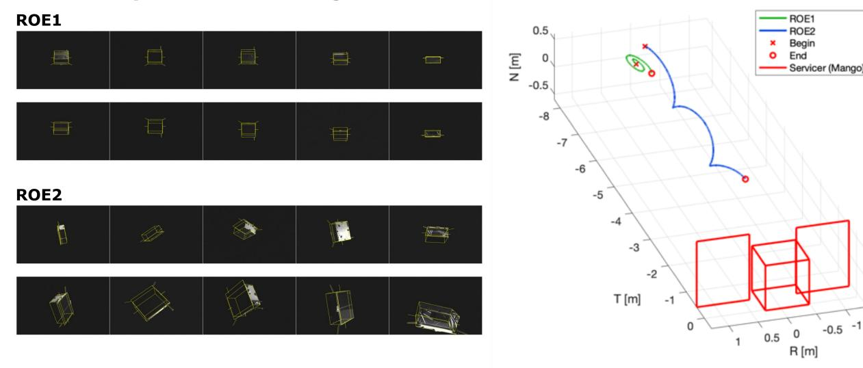
The SHIRT dataset [4] instead consists of two RPO trajectories in sun-synchronous LEO with two image domains: synthetic and lightbox. It is used for 1) offline robustness evaluation of the navigation filter with the NN as its measurement model and 2) performing OST. Note that ROE1 is more difficult as the target is located at a nearly constant distance from the camera while rotating along a single axis parallel to the image plane.
